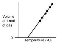
Experimentally, it is found that the line extrapolates to zero volume at -273°C. Zero degrees on the Kelvin temperature scale is defined as follows.
